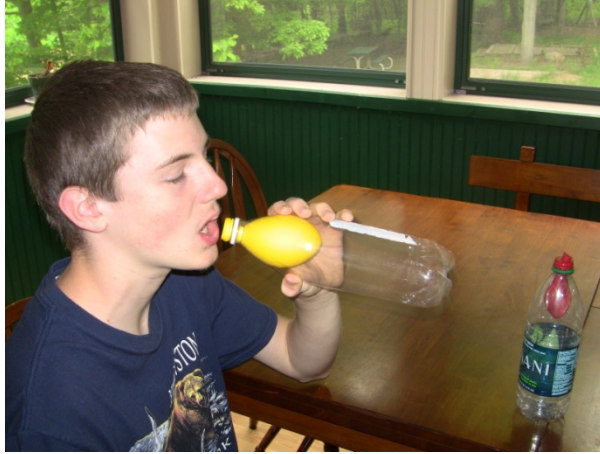
Figure 2: This is the bottle with the hole in the bottle. My air pushes so the balloon can blow up and the air in the bottle is forced out the hole.
